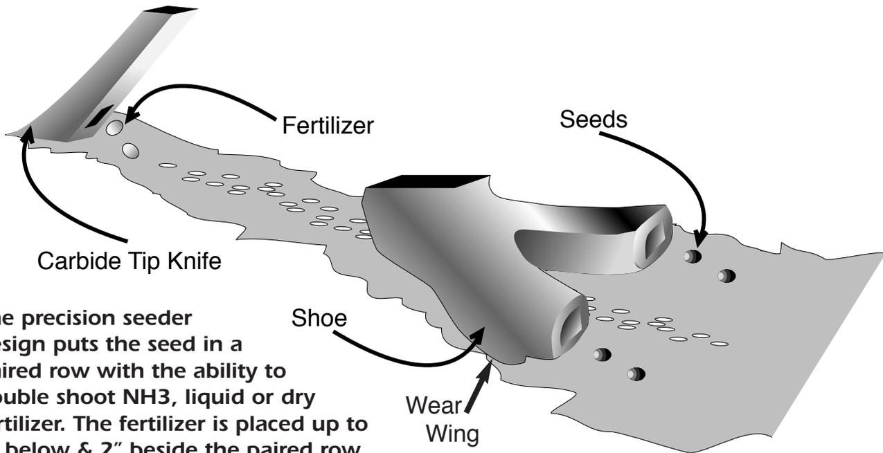
The precision seeder design puts the seed in a paired row with the ability to double shoot NH3, liquid or dry fertilizer. The fertilizer is placed up to 2" below & 2" beside the paired row.
