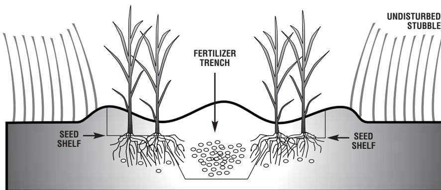
The unique knife and seed shoe combination disturbs just enough soil to help warm the seeded rows for germination. Our paired row system prepares the ground for easier seed root access to the fertilizer deposit before the weeds, thus early crop domination pushing weeds aside for cleaner, healthier crops.
